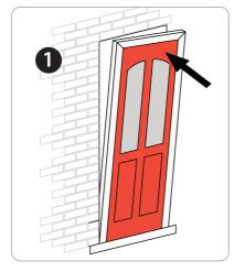
Offer complete door unit into brickwork opening.
