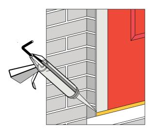
NB: Care must be taken to ensure that the drainage slots are not blocked when sealing around the aluminium wheelchair threshold.
